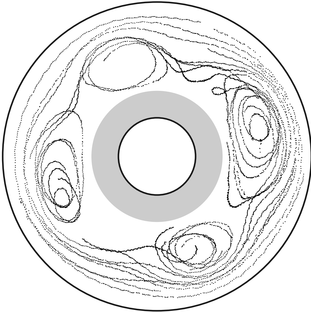
Figure 4.4: The four-vortex flow is revealed by the trajectories of 12 particles tracked for 100 s in a reference frame co-rotating with the vortices. The inner and outer circles represent the annulus boundaries, and the grey circle indicates the location of the Plexiglas barrier. (Figure from Ref. [155].)
