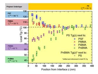
Glass – the non-equilibrium liquid state of a substance that is frozen before transitioning into a crystallized solid state – is used in applications as diverse as filtration, photovoltaic technologies, and bioengineering. Researchers and designers are finding great opportunities for enhancing glasses at the nano-level. Glasses appear to be strongly affected by their components' interfaces at the nano-level.
