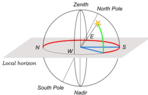
Figure 4 (from [http://en.wikipedia.org/wiki/File:Horizontal\\_coordinate\\_system\\_2.png](http://en.wikipedia.org/wiki/File:Horizontal_coordinate_system_2.png)). Horizon coordinates. Altitude is angle shown in green (between the horizon and the point of observation). Azimuth is the angle shown in red.
