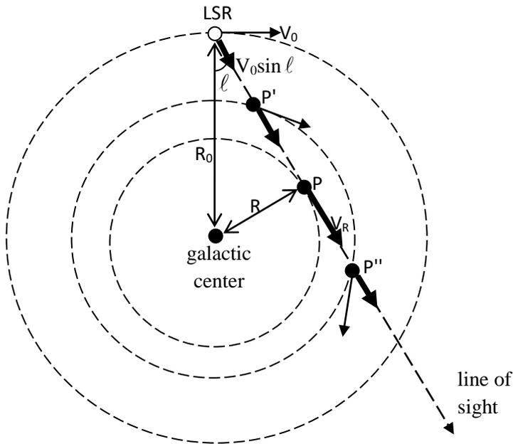
Figure 6. The local standard of rest and three hydrogen clouds (P', P, P'') moving in circular orbits around the galactic center. P is the tangent point along the line of sight. The thick arrows are line-of-sight projections of velocity.
