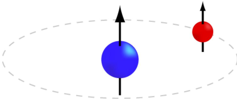
Figure 1 (from <http://en.wikipedia.org/wiki/File:HydrogenLineAntiParallel.png>). Parallel spins in the ground state. When the atom transitions to the lower-energy state of antiparallel spins, light with a 21 cm wavelength is released.
