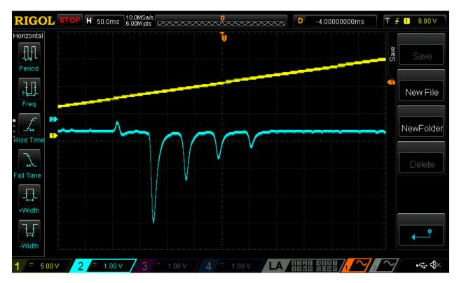
To avoid double-quantum transitions, you will need to reduce the amplitude of the high-frequency ( $\delta f$ ) voltage you are applying. The amplitude should be less than 0.5 V. Now, if you count the number of dips you can determine I! As shown at the end of the introduction, the number of magnetic field values is 2I+1. Use this method to determine I for the two isotopes of rubidium.
