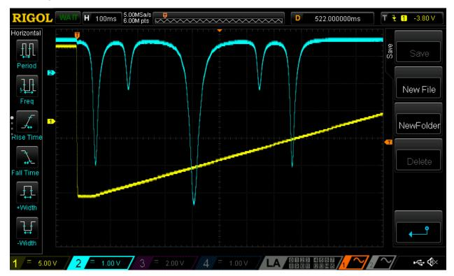
Notice the symmetry around the central dip. Recall that the central dip represents zero magnetic field. Now consider a nonzero field B. It can point in either direction along the length of the apparatus. So the regions to the right and left of the central dip indicate magnetic fields in opposite directions.
