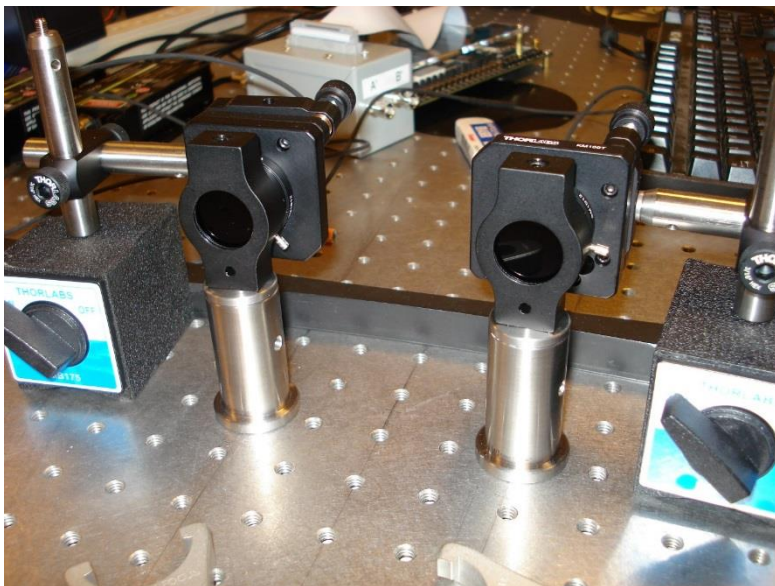
Figure 22. These optical bandpass filters block all light except wavelengths near 810 nm. These do not have to be clamped in place.
