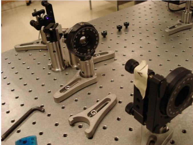
Figure 21. The half wave plate is placed between the laser and the crystal pair.
