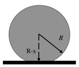
FIG. 1: Diagram of a compressed elastic sphere. The compression distance is x, so that the centerline radius has been reduced from R to R - x.
