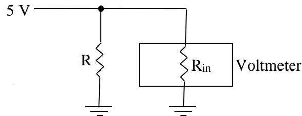
Figure 5. A voltage source connected to the parallel combination of a resistor and a voltmeter.
