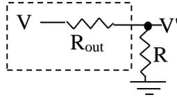
Figure 11. The "loaded" circuit (the load is the resistance between the output and ground).
