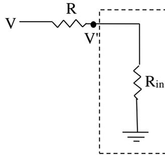
Figure 9. The circuit used to measure  $R_{in}$ .
