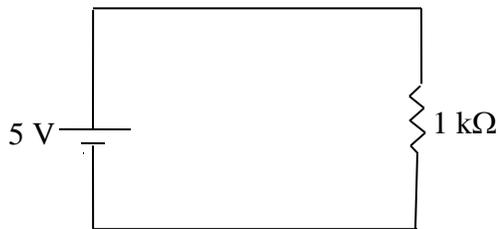
Figure 1. A circuit diagram in the style of an introductory physics textbook.
