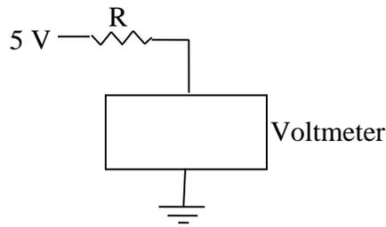
Figure 3. A voltage source connected to a voltmeter through a resistor.
