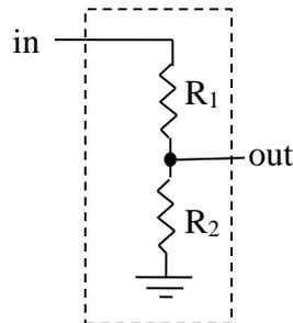
Figure 7. A circuit element known as a voltage divider.
